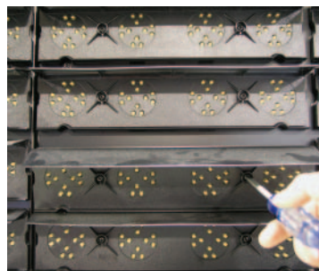
SmartStick being replaced
